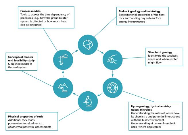
An example of a workflow for the study of geological formations, including their physical and chemical properties, to develop conceptual models to be used as the basis for dynamic modelling in energy transition projects.
