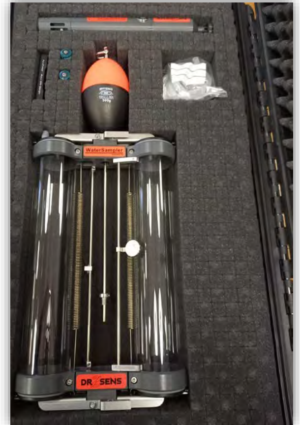
Drosens drone-borne water sampler
