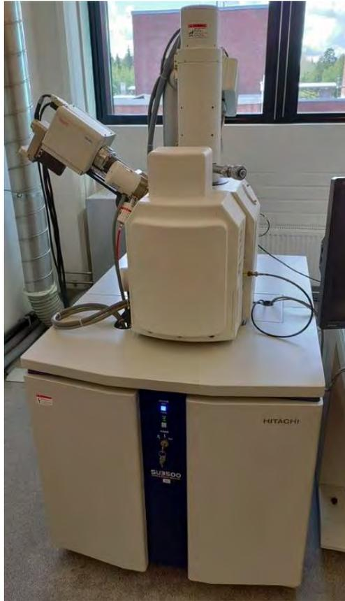
*Figure 7. SEM-EDS used to analyse the surface structure and element distribution on the sample surface.*
