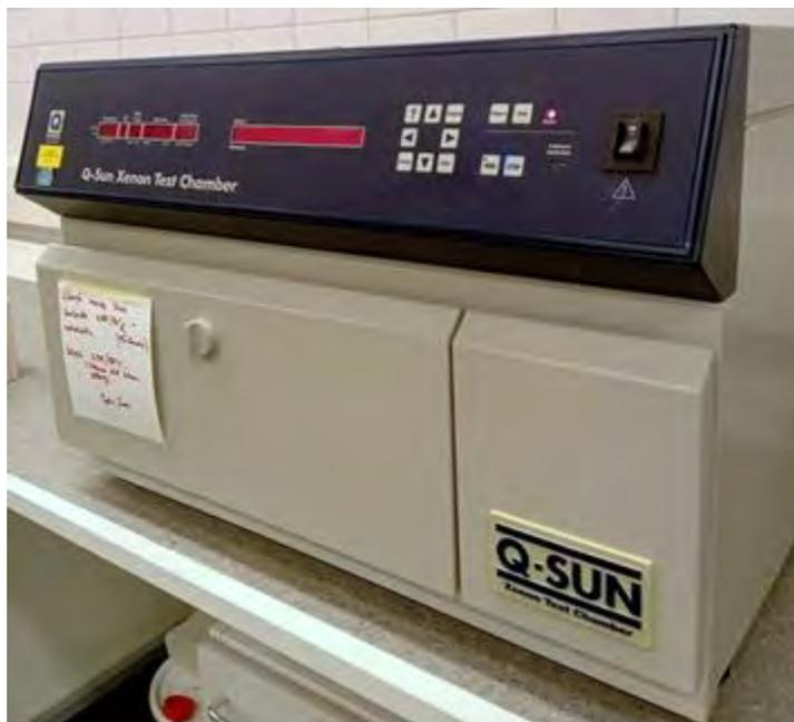
Figure 42 Q-Sun Xenon Test Chamber used for in UV light treatment.
