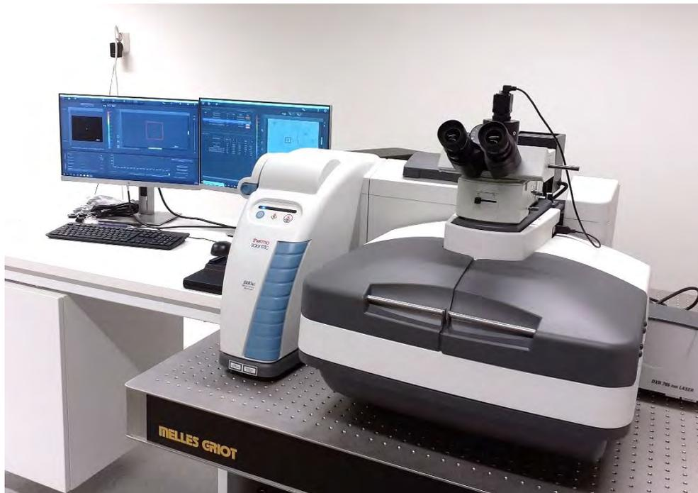
Figure 9 Mineral identification was performed with Raman imaging microscope (Thermo Scientific, DXR3xi with OMNICxi software).
