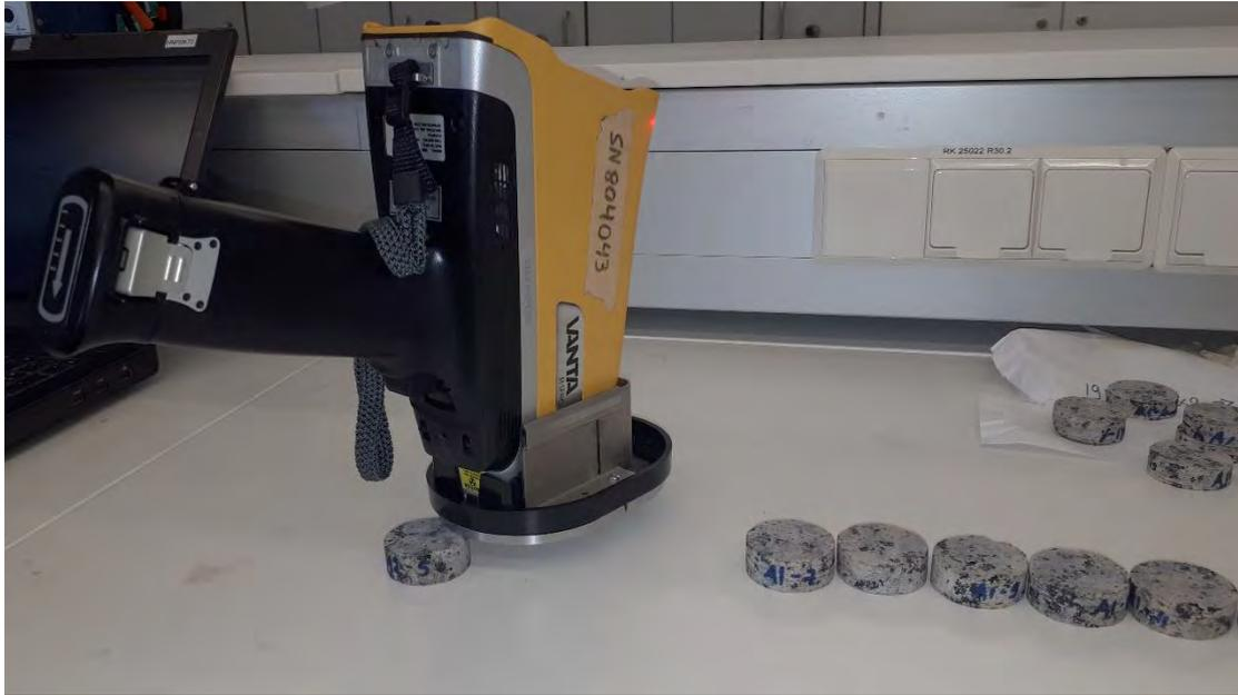
Figure 6. Hand-held device used for XRF measurements.
