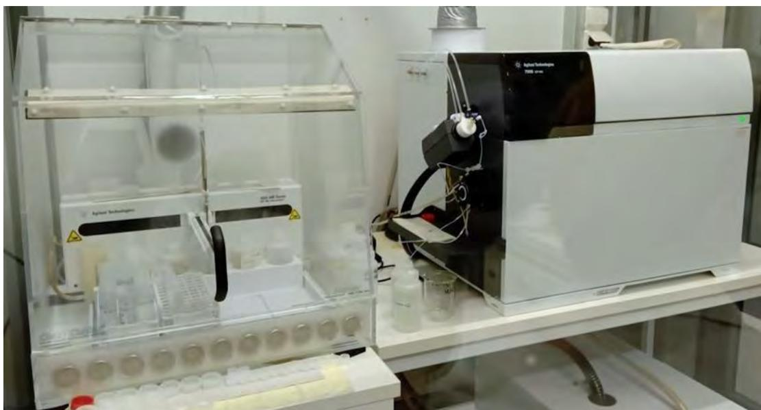
*Figure 5. Agilent Technologies 7900 ICP-MS used in examining the elements in solvents.*
