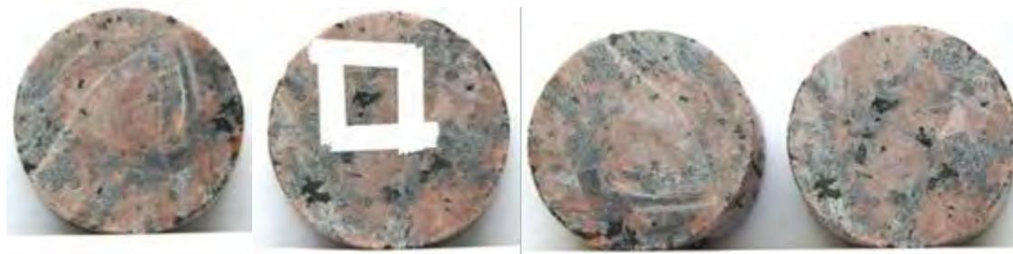
Figure 43 Samples treated with UV light treatment for 11 days. Samples U1 and U2 on the left are untreated and on the right U1 and U2 after UV light treatment.
