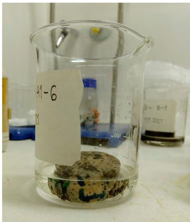
*Figure 2. Sample W-6 and approximately 50 % of its area submerged in 2 M sulfuric acid.*
