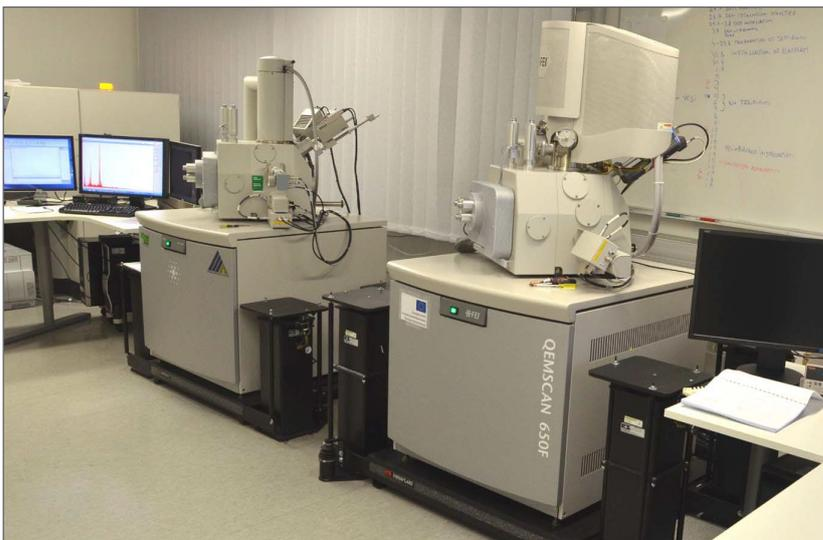
Fig. 24. GTK's process mineralogy laboratory has two pieces of SEM MLA equipment at its disposal (Torppa, 2021): FEI Quanta 650 FEG-SEM (on the right) and the FEI Quanta 600 SEM used in this study (on the left). Photo: A. Torppa.
