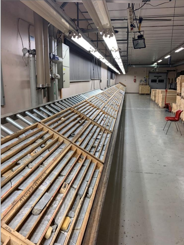
Fig. 21. One set of drill cores lifted onto the roller table for examination. Photo: J. Köykkä.
