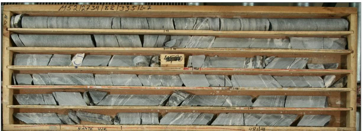
Fig. 5. Non-mineralized talc-chlorite schist with narrow quartz-carbonate veins (M273488R335).
