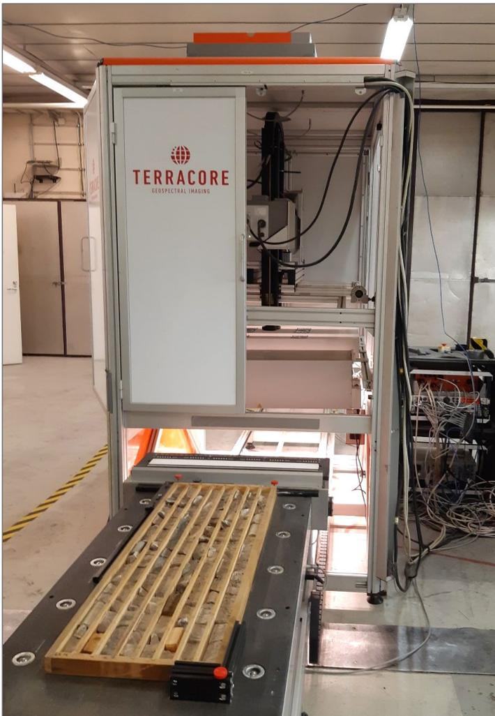
Fig. 23. The hyperspectral imaging equipment used in the study (SisuROCK Gen 2, Specim, Oulu, Finland). Photo: J. Rauhala.
