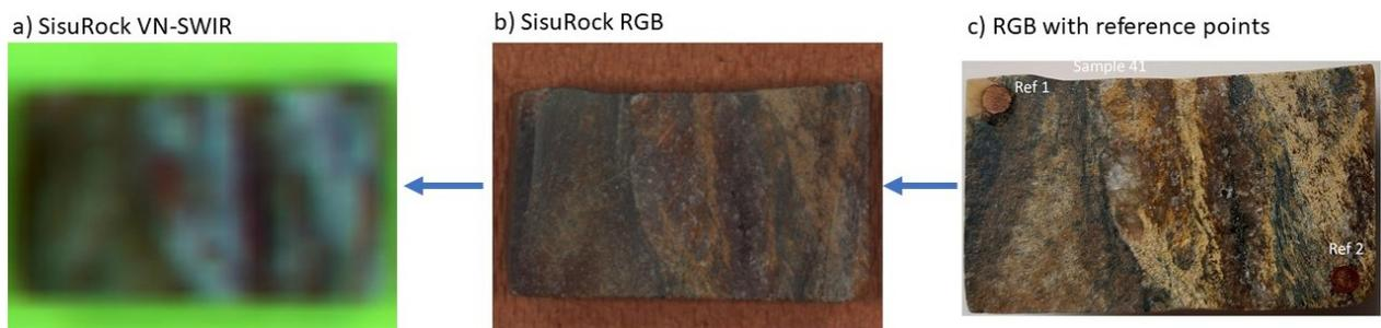
Fig. 26. Co-registration workflow of offcut HS images to RGB image with SEM-EDX/INCA reference points.
