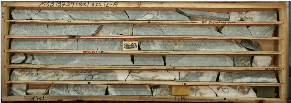
Fig. 6. Mineralized talc-carbonate-albite rock with abundant quartz-carbonate-albite veins (M273488R335).
