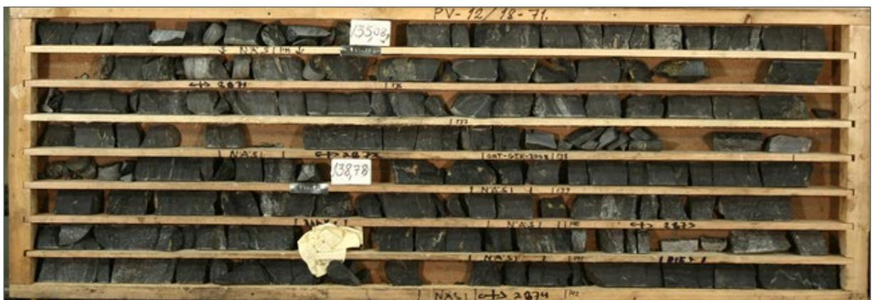
Fig. 13. Drill core tray image (PV-12), showing mineralized phyllite with narrow sulphide-carbonate-quartz dikes.
