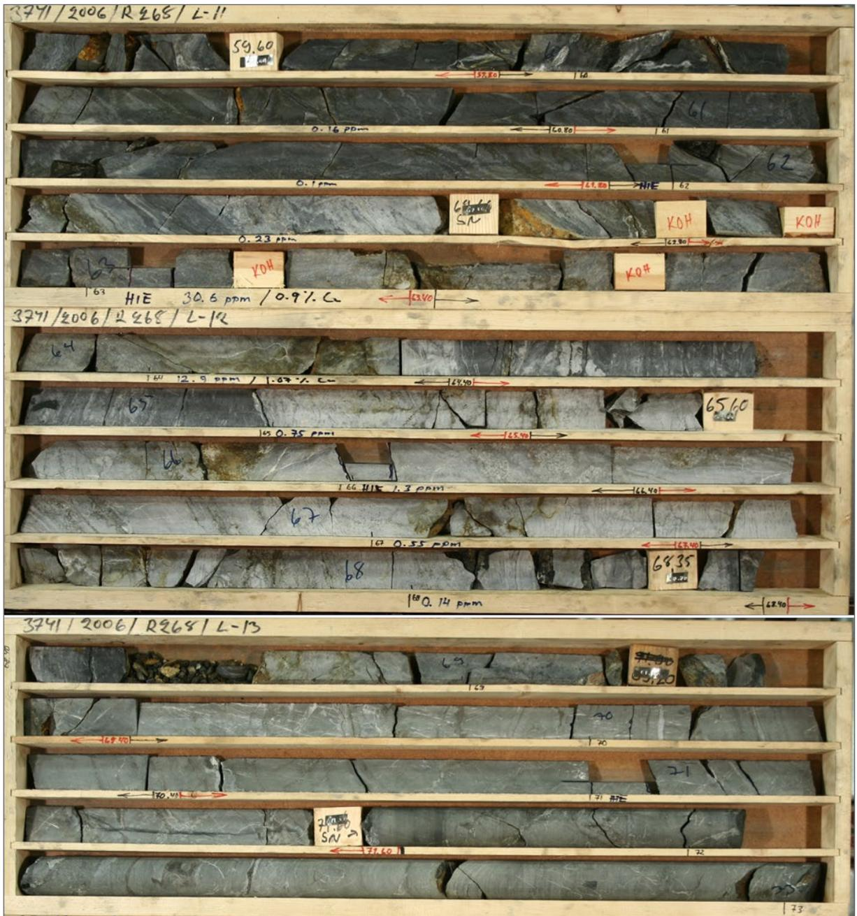
Fig. 10. Drill core tray images (M374106R268) showing the transition from the less mineralized dark biotite-sericite altered mica schist to the highly Au-mineralized quartz-albite-rich rock. Also note the sharp contact of mineralization and alteration with mafic volcanic rock on the foot wall.
